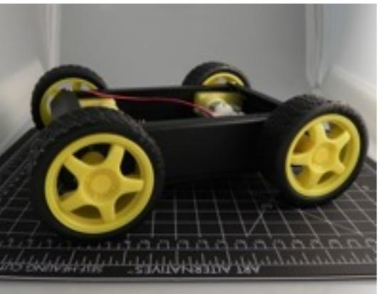
*4WD Arduino Compatible Mobile Platform
